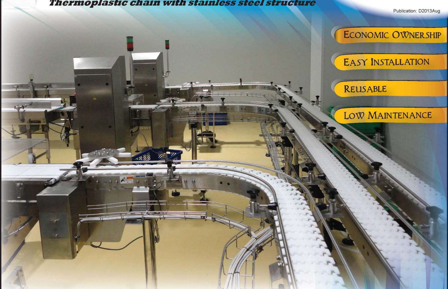
**MODU System** Stainless Steel Conveyor provides a structural stainless steel conveyor which uses our standard multi-flex plastic conveyor chain. The stainless steel conveyors are designed with similar concept as aluminium conveyors. MODU Conveyor's modular design comprehends trouble-free line configurations, site installation and maintenance making them cost effective and simple to use. Conveyors be reconfigured or assembled in quite a less time using simple hand held tools.
